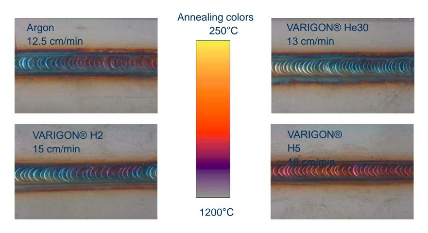
TIG manual fillet weld on 4.0 mm thick 304, filler ER 308 L Si, Ø 2.0 mm
